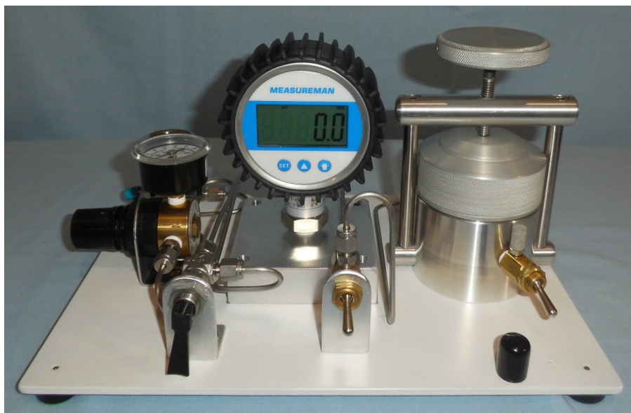
Fig. 1. Illustrative version of the Edu-Pyc 101 Pycnometer
