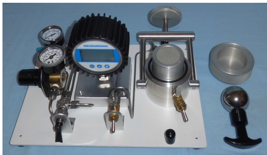
Fig. 2. Opened sample chamber with the sample holder placed inside.
